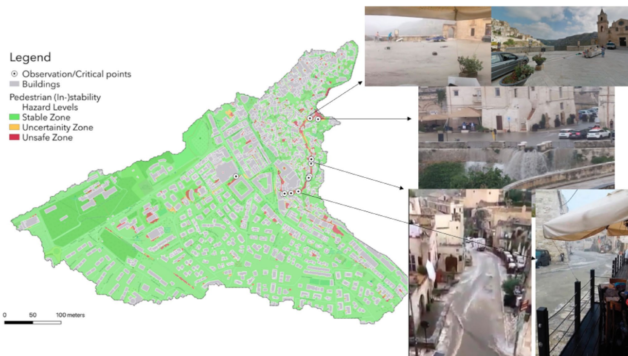
Fig. 6 Assessment of pedestrian stability and instability hazard levels in the “Sasso Caveoso” urban basin during the 2019 flood event
