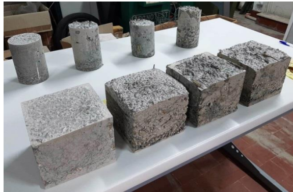
Fig. 1 Cubic and cylindrical samples for the laboratory tests
