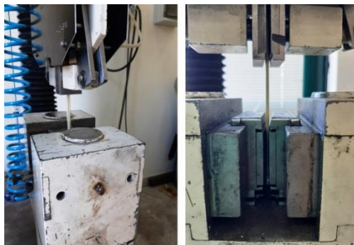
Fig. 2 Tensile tests on Arundo donax fibers: front view (left) and side view (right)
