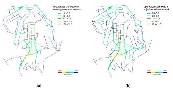
**Figure 19.** (a) Topological connectivity of existing pedestrian route network; (b) topological connectivity of project pedestrian route network.
