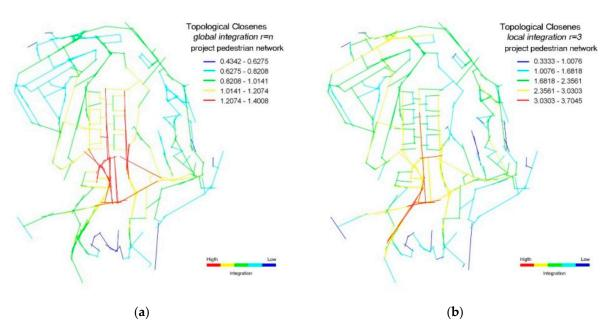
**Figure 17.** (a) Global Topological integration (r = n) and (b) local topological integration (r = 3) calculated on the project network.
