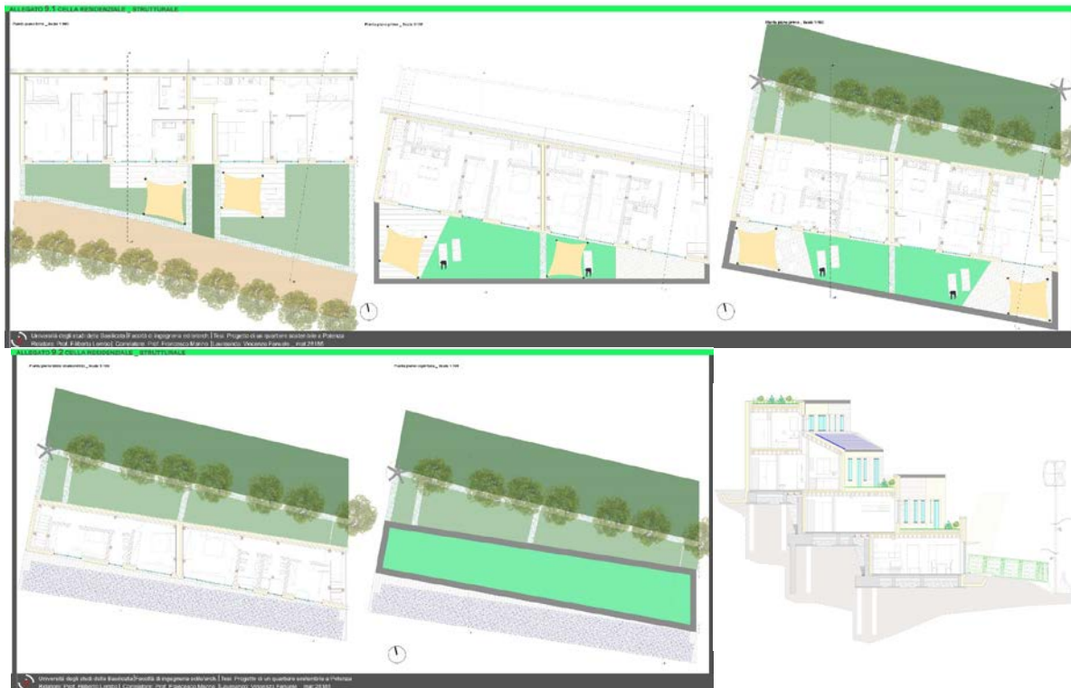
Figure 9. Residential cell type, distributed on three levels (top view) and a maisonette (bottom left) for a total gross area of 600 m 2 ; roof plan (bottom center) and cross-section (bottom right)
