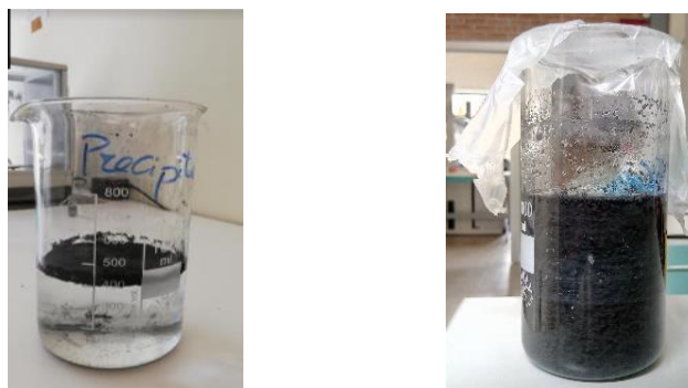
Fig. 45 Picture of TPEG in the water before sonication treatment (on the left) and after 50 hours of sonication treatment (on the right).
