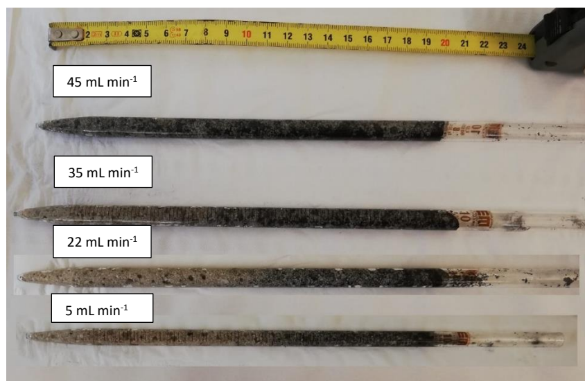
Fig. 61 Pictures of soil chamber after TPEG injection. “Hydro-soluble” TPEG’s solution was injected into soil-chamber at different flow rate (5, 22, 35 and 45 \text{mL min}^{-1} ).
