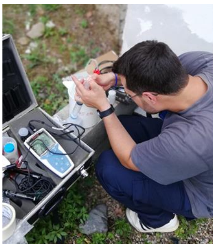
Figure 25 – in situ filtration and measurement of physico-chemical parameters of a water sample.
