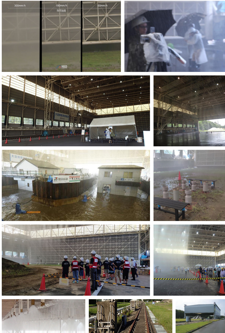
Figure B.4: Experiments in the NIED rainfall simulator.
