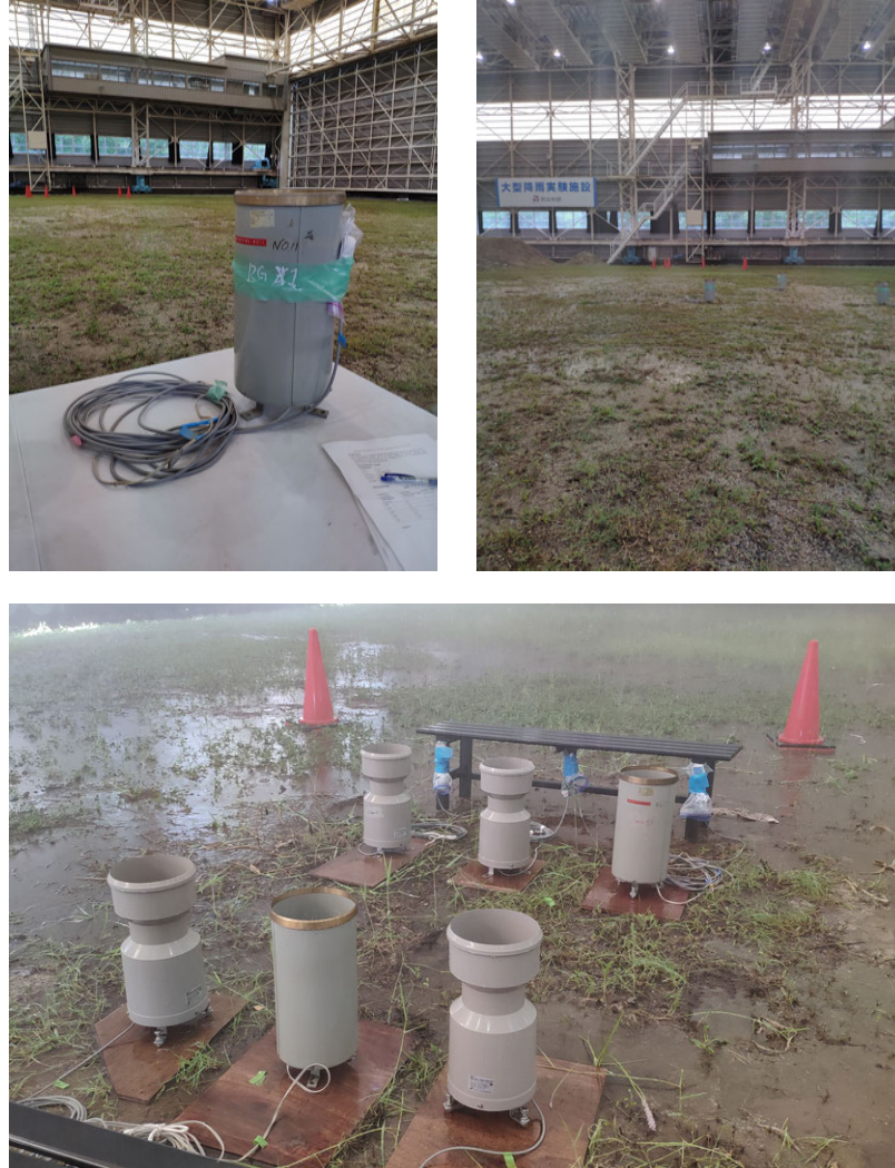
Figure 5.5: Rain gauges used for checking nominal rain intensity.
