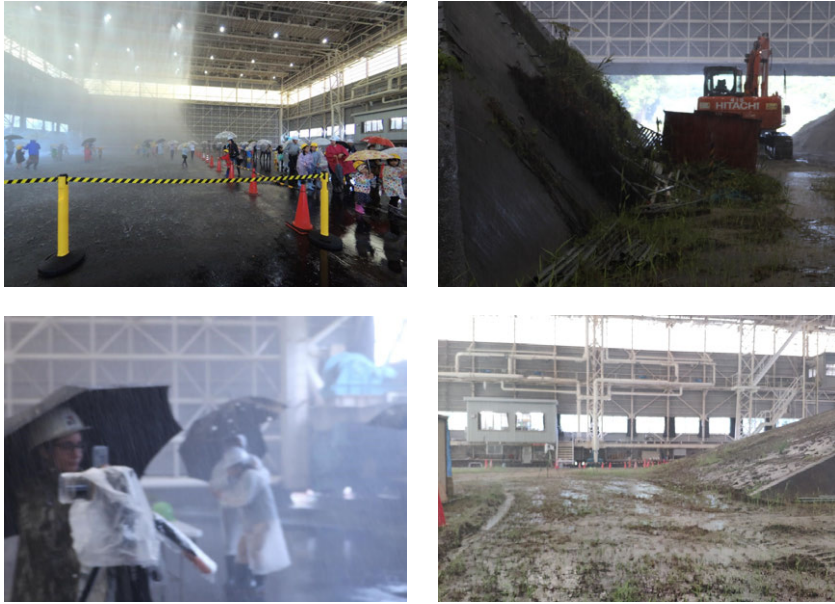
Figure 5.4: NIED Large-scale Rainfall Simulator experiments.
