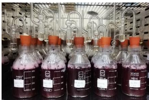
Figure 4.15| Mixed fermentations in grape must in flasks closed with a Müller valve filled with sulphuric acid.
