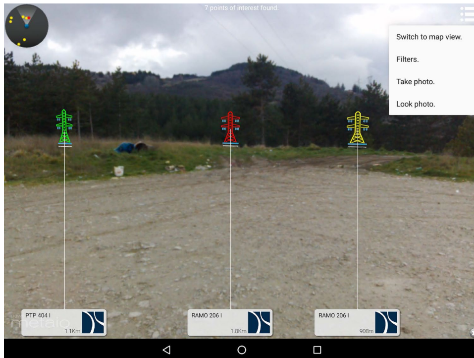
Fig. 4 The augmented reality application for electrical power lines. The points of interest visualize the position of three pylons, with the colours indicating the status of each pylon. The yellow circle in the radar display (top left) indicates the positions of pylons, and the blue circle is the mobile device. (Colour figure online)
