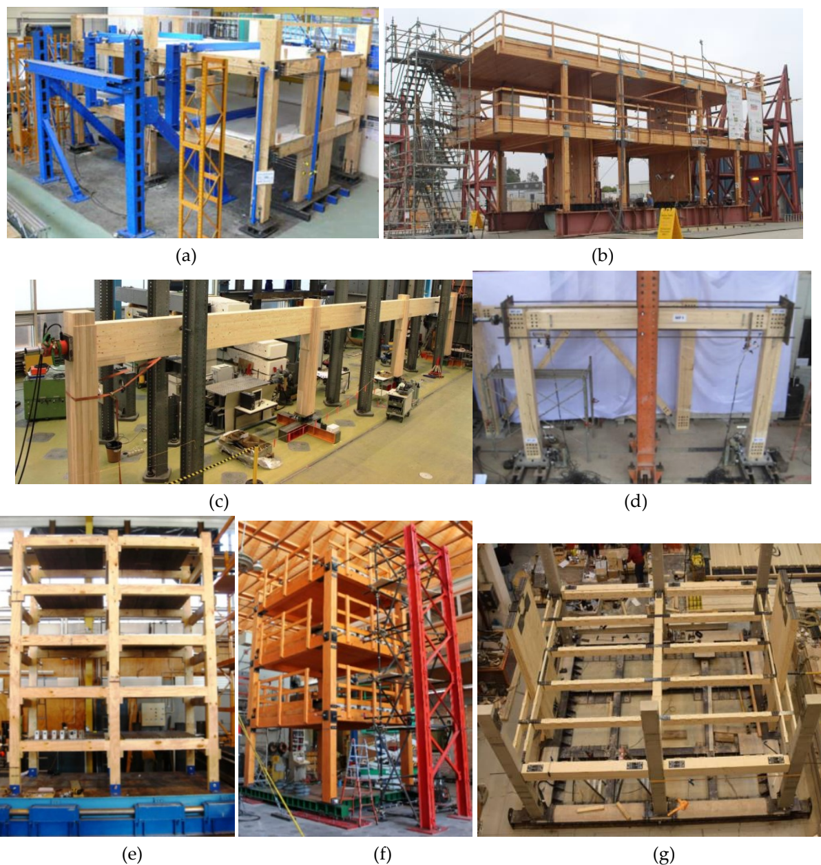
Figure 8. Experimental testing on: (a) LVL frame with post-tensioning and post-tensioned rocking walls with UFPs (Newcombe et al. 2010) [10]; (b) mass timber building with post-tensioned CLT rocking walls (Pei et al. 2016) [11]; (c) bidimensional post tensioned frame (Wanninger and Frangi 2016) [72]; (d) post-tensioned portal frame (Xiong et al. 2016) [73]; (e) post-tensioned LVL timber framed building (Pino et al. 2010) [74]; (f) post-tensioned glulam timber framed building with dissipative rocking Pres-lam project UNIBAS (Di Cesare et al. 2017) [13]; (g) timber-concrete test building – SERA project (Pamapanin et al. 2020) [75].
