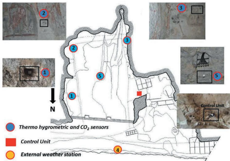
**Figure 3.** Plan of the Crypt. The figure also reports the sensor localization scheme of the monitoring system. Sensors 1 and 2 measure T, RH and CO<sub>2</sub> close the paintings showed in Figure 2.
