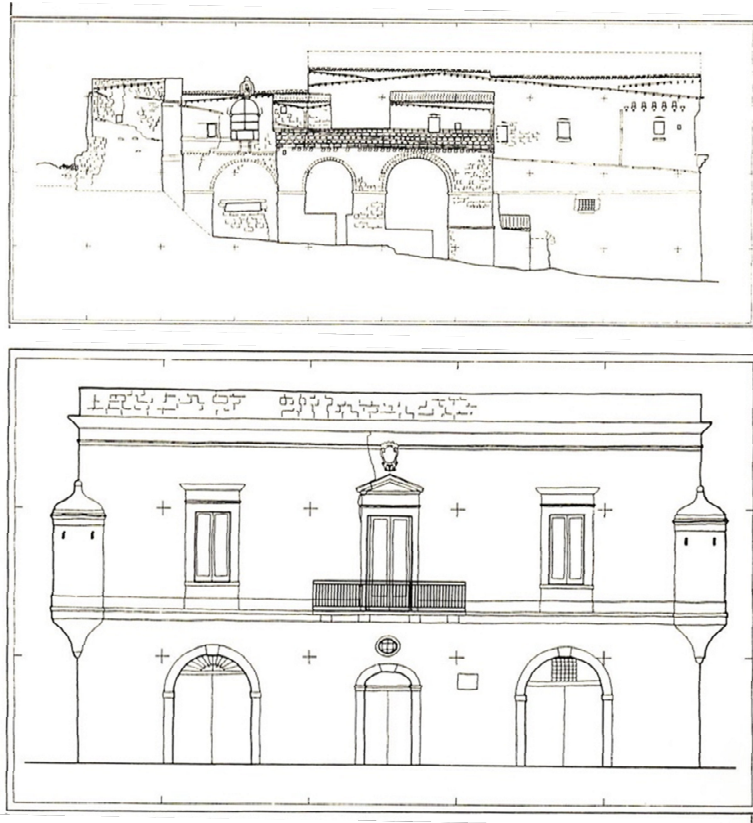
Fig. 1 Façades of masserie located in the Basilicata region (southern Italy), surveyed through terrestrial photogrammetric techniques [15].
