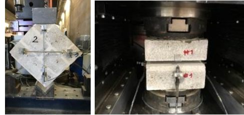
Figure 3. Details of tests on masonry assemblages: (a) Diagonal shear test; (b) Tensile test setup
