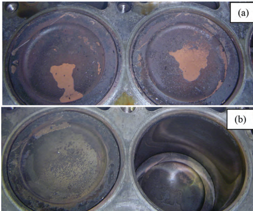
Figure 9: The cylinder faces of internal combustion engines after the test run: (a) control car (without the additive); (b) testing car after application of the additive.
