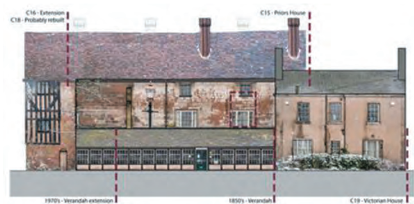
Figure 9: Photo elevation and analysis of West elevation.
