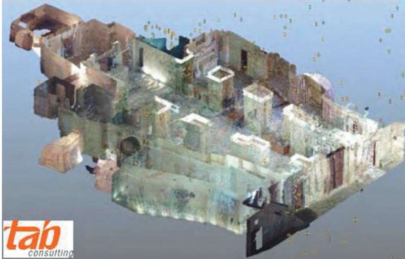
Figure 5: Axonometric section of the complex point cloud of the church of San Pietro Barisano.
