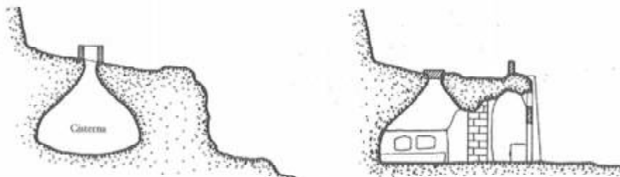
Representation of the evolution of the type of housing from underground cistern a hypogeum. LAUREANO P., 1997, pg. 118.
