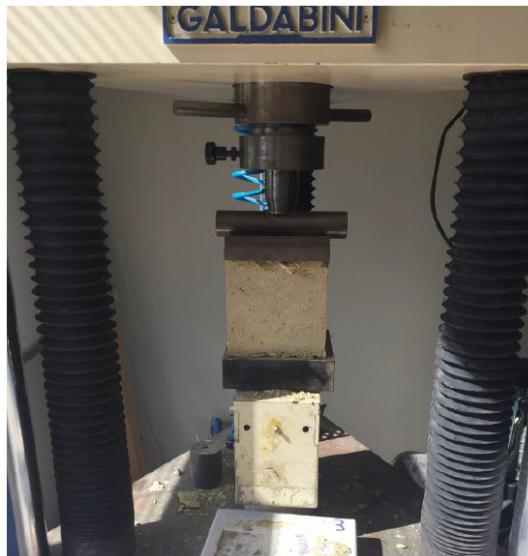
Figure 5. Compression test on an adobe bricks.
