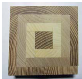
Figure 1: CCLT lath (ash, aspen, birch, ash; from inside to outside ), specimen S 01 KK2.
