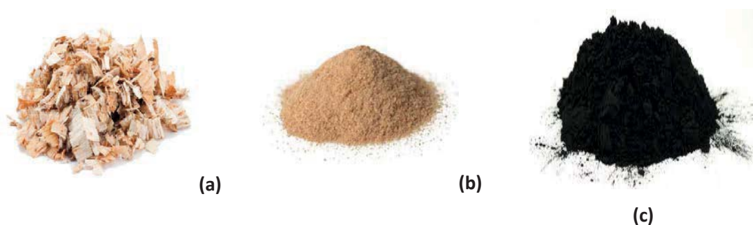
Figure 1: Images of (a) Sawdust; (b) Powdered sawdust; (c) Sawdust-based AC.
