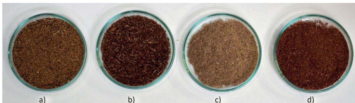
Figure 1: Overview of the various wood materials a) beech, b) pine, c) black locust, d) larch.
