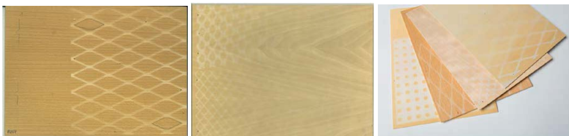
Figure 1: Samples of UV-modification on poplar and beach wood by using different mesh masks and samples with the special transition pattern thanks to inclination of the mask.
