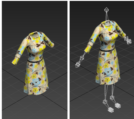
Fig. 3. A 3D item of clothing without (left) and with (right) the virtual skeleton.
