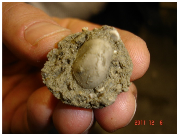
Figure 1. Example of newly formed aggregate from returned concrete
