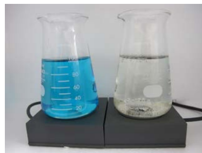
Effect of the treatments on the degradation of methylene blue. Left: 10mM \text{H}_2\text{O}_2 alone and right: 10mM \text{H}_2\text{O}_2 and 0.1 mM of Fe as catalyst made using coffee grounds.
