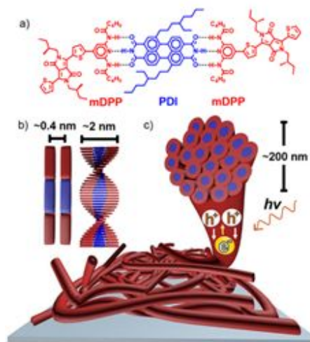
Figure 1. a) Chiral mDPP donor (red) and the PDI acceptor (blue) form 2:1 aggregates as a result of H-bonding. b) \pi -stacking orthogonal to the H-bonding creates donor-acceptor superstructures with helical chirality. c) Drop-casting of a 2:1 mDPP:PDI solution results in films comprised of hierarchical ropes whose fibers are the chiral superstructures that contain \pi -channels for transport following photoinduced charge separation.
