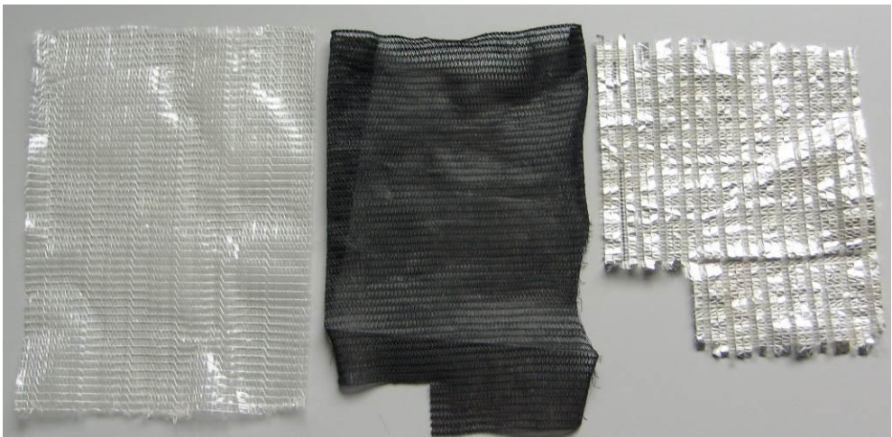
Figure 1 The three analysed plastic nets: white net (left), black net (centre), aluminized thermal screen (right).
