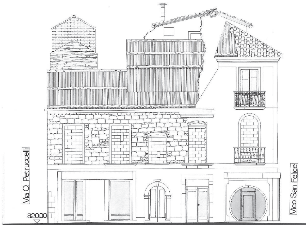
Fig. 6: Survey's drawing of a building on via Pretoria. The survey becomes an important document of the damages on the manufact after the earthquake of 1980 (from DE NUCCI Alberto, TOLLA Enza, 1988).
