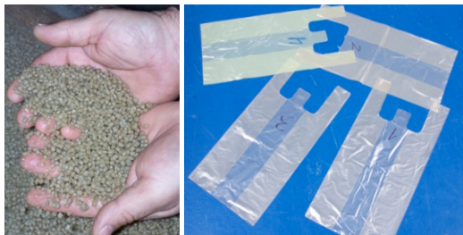
Figure. 1 Granulated material and new, regenerated films
