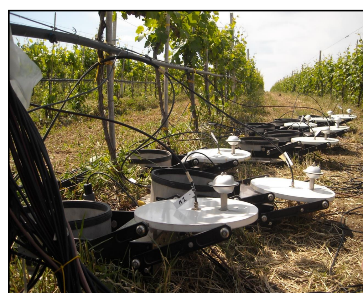
Photo 2. System of total soil respiration measurements.
