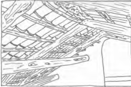
Fig. 4 Internal structure of a typical roof in the Vesuvian area (Image: Archivio Mollo/DIC)
