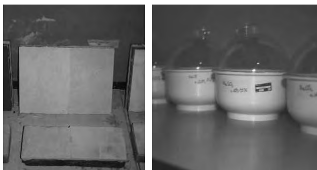
Fig. 3,4 - Pictures showing the reproduced traditional plasters and the experimental facilities used for the determination of the sorption isotherms
