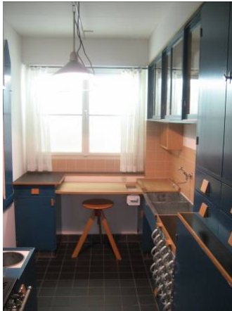
Fig. 4 The Frankfurt kitchen was designed for social housing in Frankfurt. It was the first mass-produced kitchen with a comprehensive design. Note the adjustable chair.
