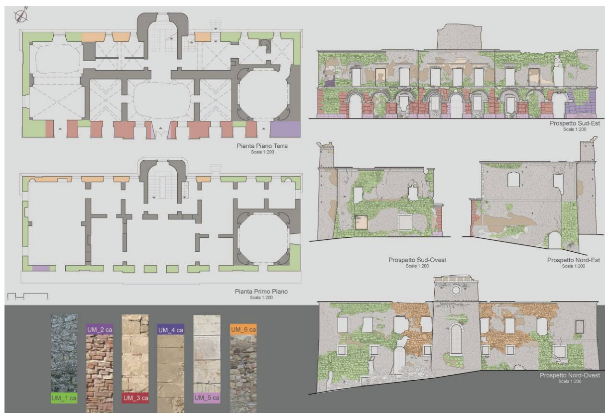
Fig. 4: Analysis of masonry panels of the Casino of the Countess in Campomaggiore.
