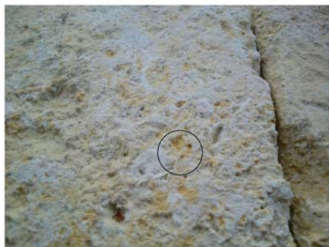
Figure 10. Caloplaca flavescens (Huds.), on calcarenite stone examined after 3 months of exposure to the atmosphere action.
