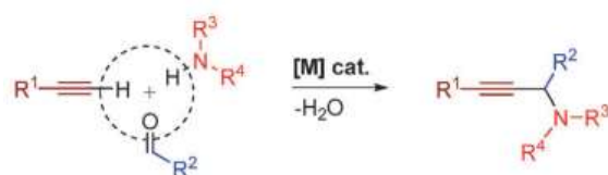
Scheme 4 – A 3 coupling reaction (Aldehyde–Alkyne–Amine)
