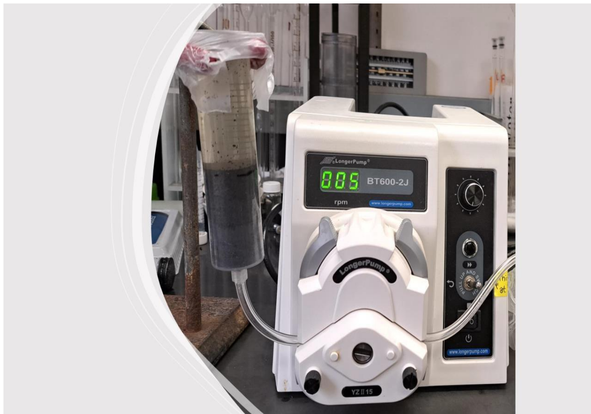
Fig 3.3. Column system and connection to a pump for removal of dissolved oil
