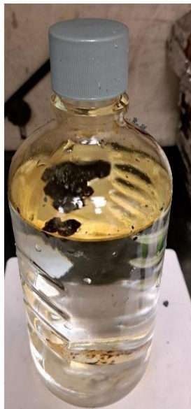
Fig 4.49. Floating oil removal experiment by EG powder (6 g oil, 180 mg EG)
