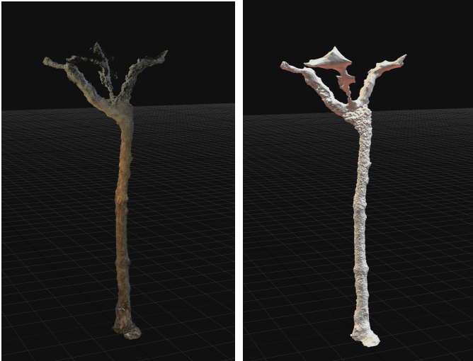
Fig. 3: The point cloud and the mesh of the trunk reconstructed using Reality Capture. It was placed in the corresponding tree location of the ATD.
