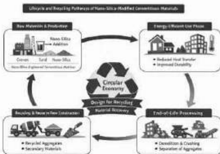
Figure 3. Lifecycle and recycling pathways of nano-silica-modified cementitious materials.
