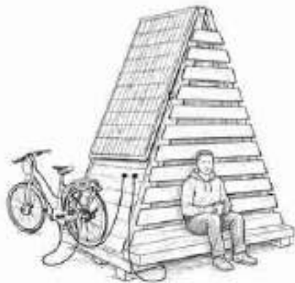
Figure 3. View of one of the devices supporting cycling mobility, designed for charging and temporary storage of electric bicycles, as well as for powering small electronic equipment.
