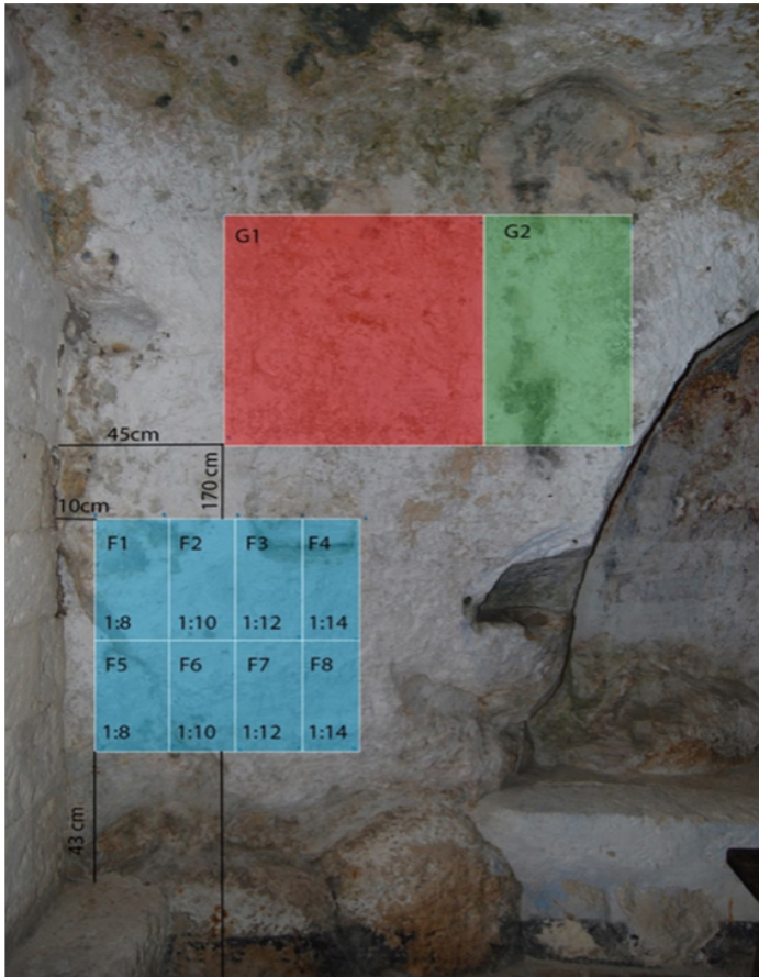
Figure 14. Treatments of sample area in the interior surfaces of the church of Madonna dei Derelitti with the pilot products POLYRESTP2(F1-F4) and AC012 (F5-F8) and commercial ethyl silicate products (G1-G2).
