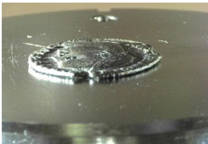
Fig. 3. The coin loosely positioned on the sample plate in the Sample Environment.
