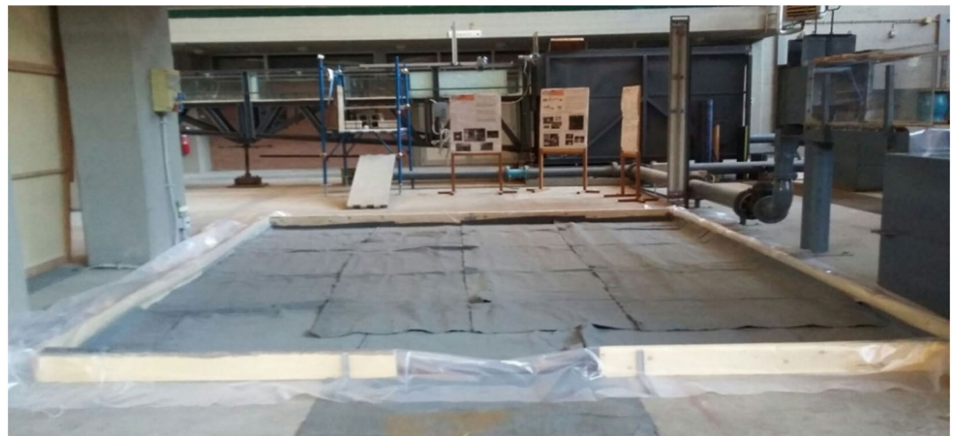
Figure 9. Empty wooden basin utilized to simulate the sandy alluvial floodplain in the Laboratory of Hydraulics and Hydraulic Constructions at University of Basilicata.
