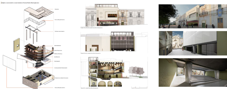
Fig. 9. Axonometric exploded view, new shell with different uses; Project drawings for the restoration of the Mastrogiacomo Cinema-Theatre; Project views.
