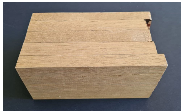
Figure 3 | Photo of a laminated conditioned Quercus cerris glulam specimen.
