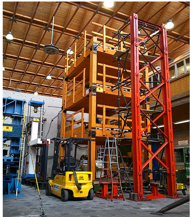
Figure 17 | SisLab Unibas: real-scale wooden building under seismic test.
