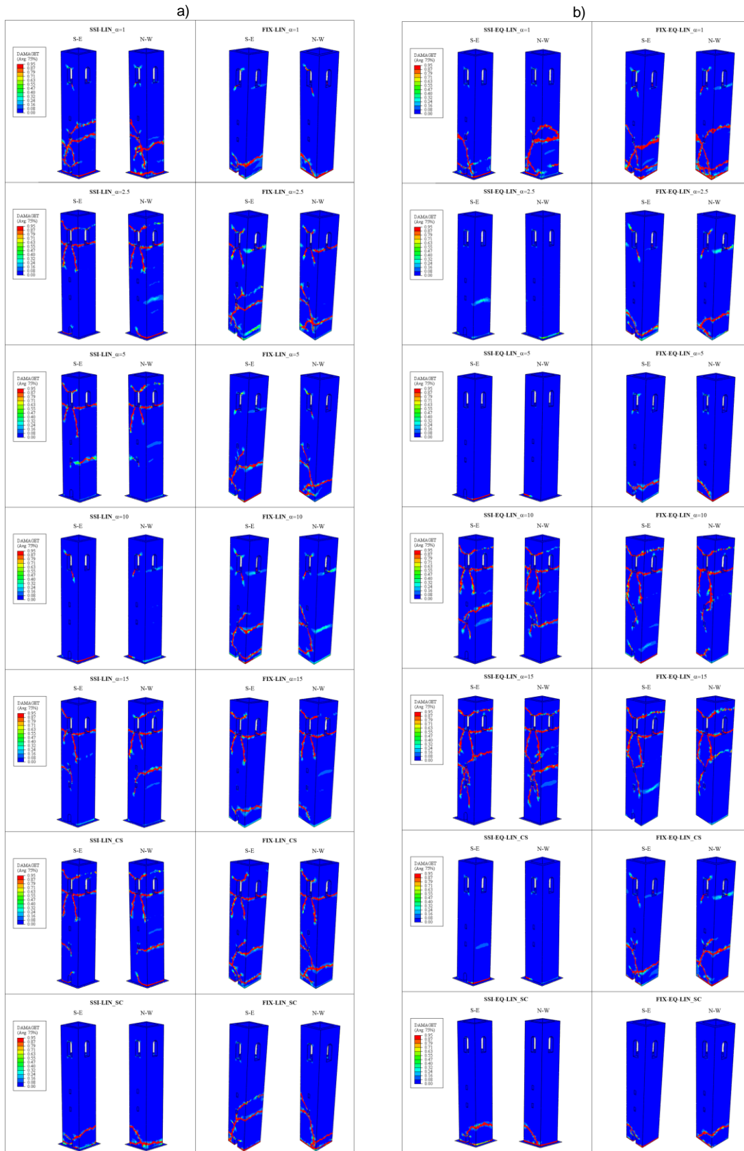
Figure 4. Tensile damage contours at the end of the seismic action for the a) LIN and b) EQ-LIN analyses, compared with the corresponding fixed-base solution.
