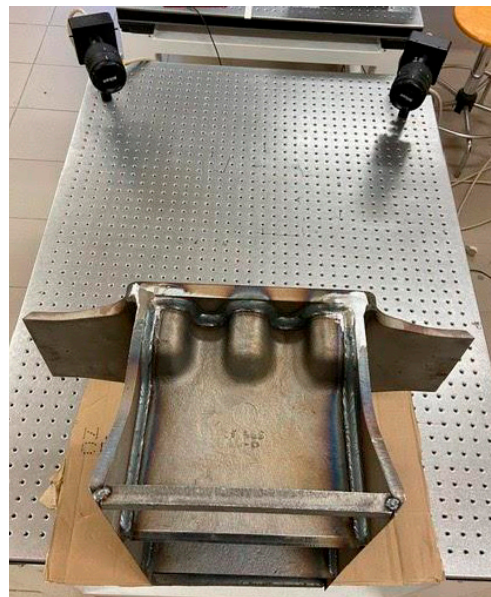
Figure 2. Layout of the stereo-DIC system used to measure welding-induced distortions on the front plate of the traction frame subassembly of a train bogie bolster.
