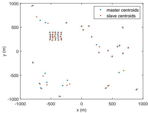
Fig. 3. Centroids detected and coupled for the Carabas-II master and slave images.
