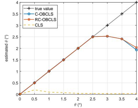
Fig. 4. Estimated rotation angle for Carabas-II SAR images.
