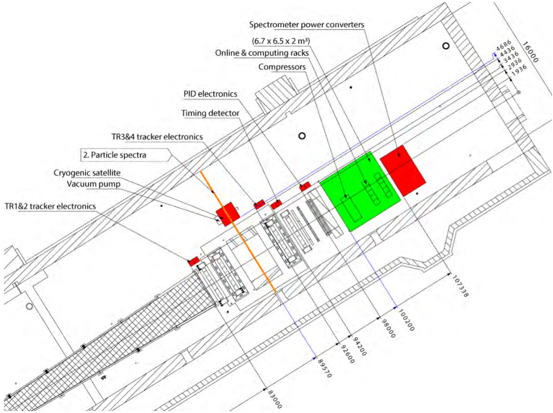
Figure 31: The integration layout shows the cryogenic satellite in the corridor next to the spectrometer magnet. Excerpt from the SHiP "Input layout for R2E and background studies", DWG SPSXXSHIP0002 EDMS 3301751 v1.2 dated 25.08.2025.
