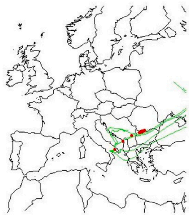
Fig. 7. Output of the procedure detecting the influence of biomass burning on EBC concentrations measured on October 14, 2018. The 500 m a.g.l. back trajectory, moving within the boundary layer, intercepts many fires.
