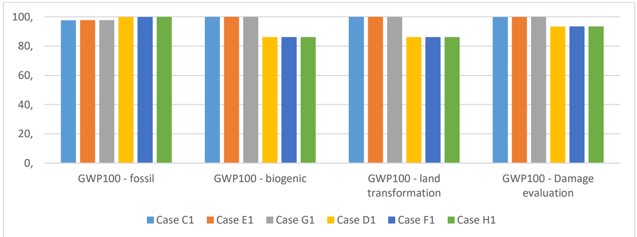
Figure 40: Comparative Global Warming Potential between MAP-Vacuum (RM Case C1-E1-G1 vs PM Case D1-F1-H1) across different storage time intervals (30-60-90 day), using the IPCC 2021 GWP100; (FU: 1 kg Mozzarella).
