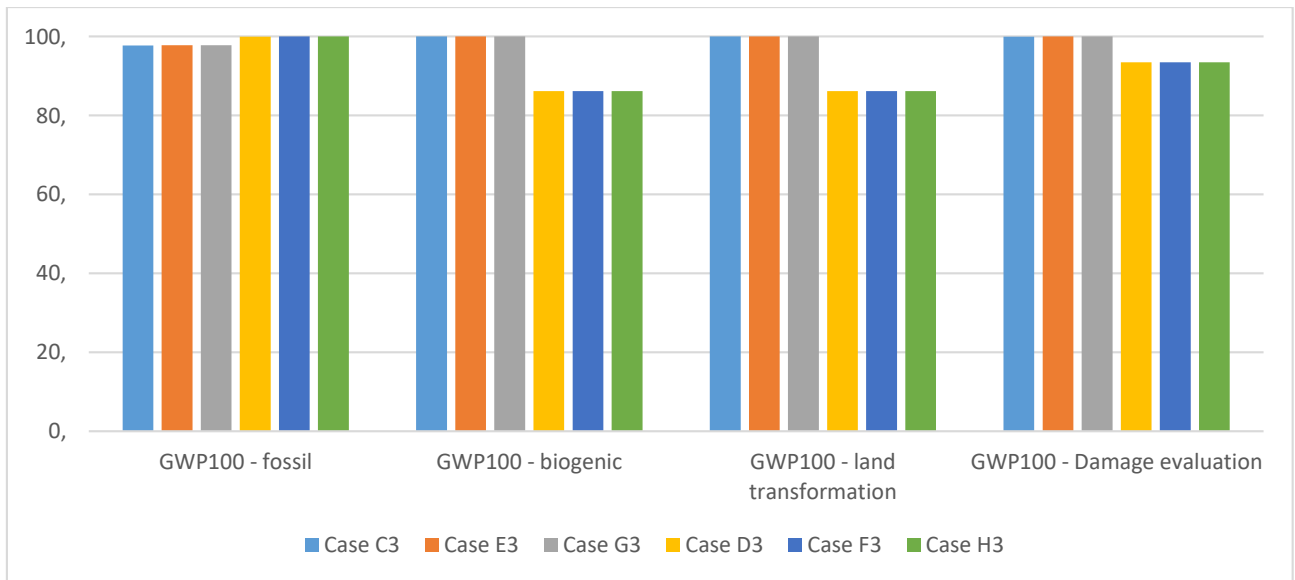
Figure 77: Comparative Global Warming Potential between MAP-Nitrogen (RM Case C3-E3-G3 vs PM Case D3-F3-H3) across different storage time intervals (30-60-90 day), using the IPCC 2021 GWP100; (FU: 1 kg Mozzarella).
