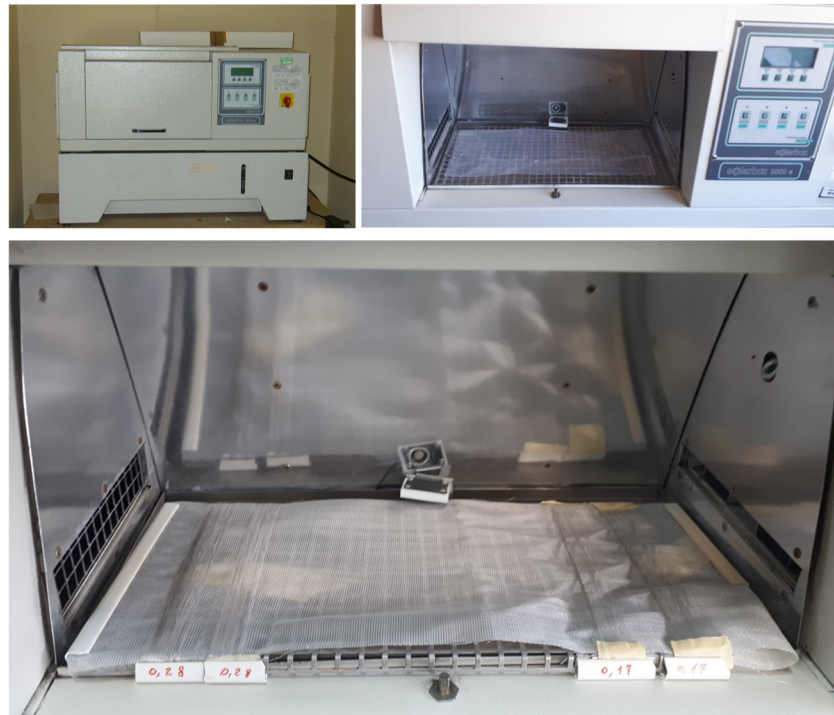
Figure 2. CO.FO.ME.GRA SolarBox 3000e artificial ageing chamber.
