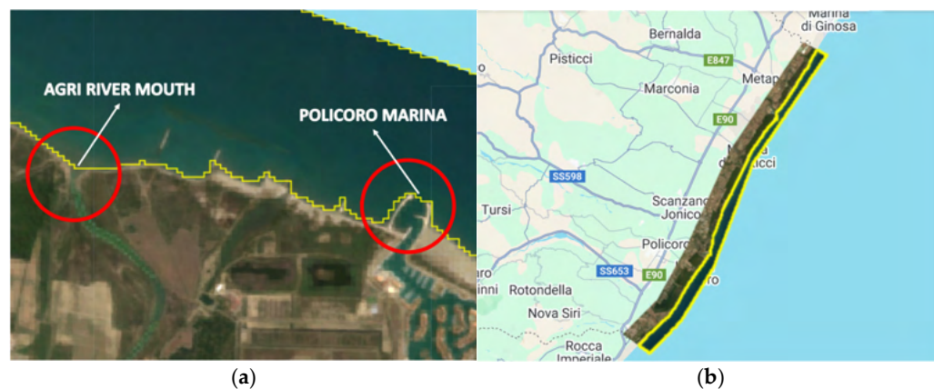
Figure 4. Post-processing of the MNDWI–Otsu water mask and sea-polygon selection. (a) Examples of morphological opening used to remove narrow, spurious water connections at the Agri River mouth and the Policoro harbour inlet. (b) Example annual composite (2025) over the coastal strip and corresponding sea polygon extracted (outlined in yellow) from the cleaned water mask, retaining only the largest contiguous water body (Ionian Sea) for shoreline delineation.
