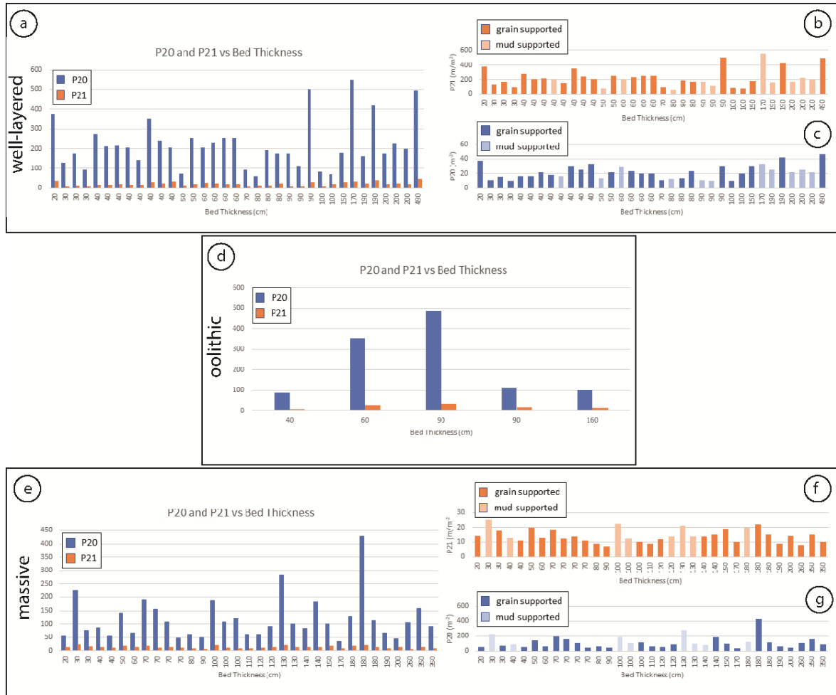
Figure 2. 14 ) Bed thickness vs P20 and P21 values for (a) well-layered carbonates; (d) oolitic carbonates; (e) massive carbonates. (b) Bed thickness vs P20 for the mud-supported carbonate, in which the grain supported and the mud supported beds are highlighted; (c) bed thickness vs P21 for the mud-supported carbonate, in which the grain supported and the mud supported beds are highlighted; (f) bed thickness vs P20 for the massive carbonate, in which the grain supported and the mud supported beds are highlighted; (g) bed thickness vs P21 for the massive carbonate, in which the grain supported and the mud supported beds are highlighted.
