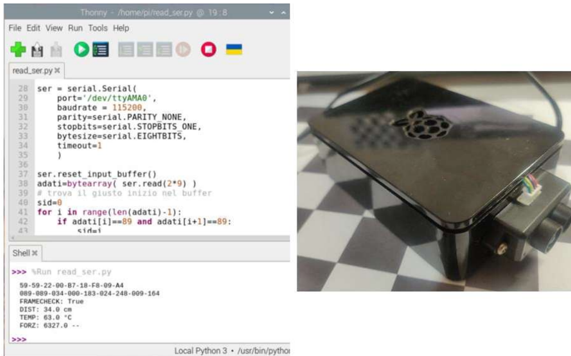
Figure 4.22. Run of the Python script to test for the serial connection of the LiDAR sensor and the LiDAR device connected to the Raspberry Pi3 hardware.
