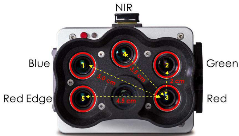
Figure 2.8. Location of the optical lens of the Micasense RedEdge P sensor and relative pose of the spectral bands (B, G, NR, RE) to the R band, with distance from the reference lens (cm).
