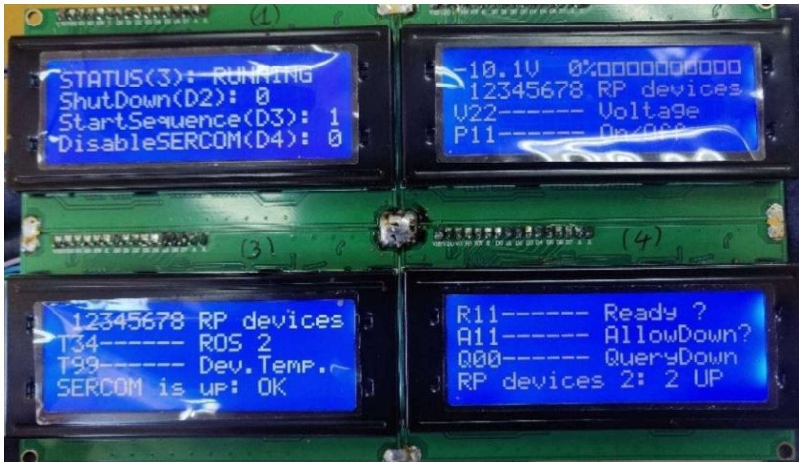
Figure 4.36. Initialization and runtime status screens displayed on the four I 2 C-connected LCD modules of the Overall Master Control (OMC), showing system version, device checks, ROS 2 communication status, power supply information, and safety-related flags.
