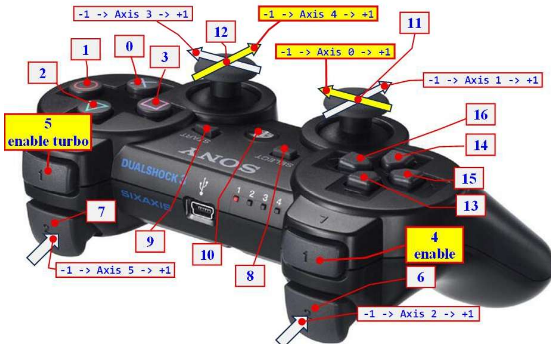
Figure 4.38. Buttons and Axes mapping for the PS3 controller.
