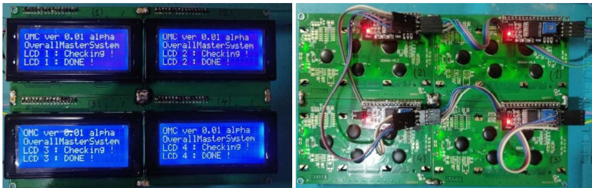
Figure 4.35. LCD-based system status visualization implemented on the Overall Master Control (OMC). The four I 2 C-connected displays provide real-time feedback on system initialization, device availability, ROS 2 communication status, power conditions, and safety flags, enabling local supervision of the distributed robotic architecture.
