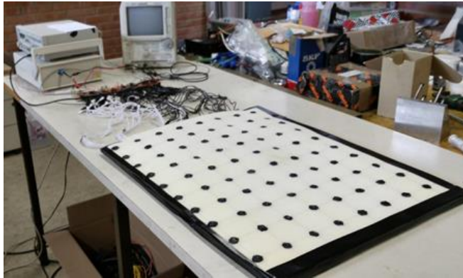
Fig. 7. A view of the device equipped with the signal generator, the amplifier and an oscilloscope for monitoring the driving signal
