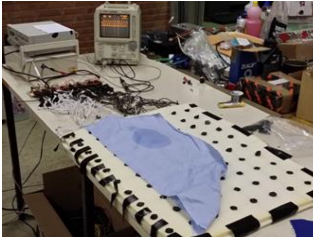
Fig. 17. Drying test of fabric with an area soaked in distilled water (darker area on the fabric lying on the instrumented mat)
