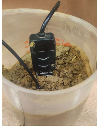
Figure 3.14 Placement of moisture and temperature probes in the soil sample: The SEN0308 probe is inserted vertically at a depth of 15 cm, while the DS18B20 sensor is positioned at 5 cm depth. This arrangement allows synchronous monitoring of soil moisture and temperature parameters during the natural soil drying process.
