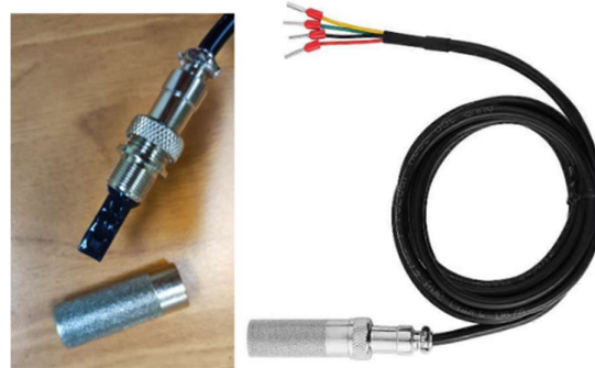
Figure 3.6 SHT10 sensor based on CMOSens ® technology (left) and version integrated into a probe with porous metal casing for field applications (right).
