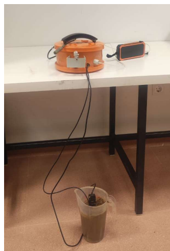
Figure 3.15 Placement of the complete monitoring system: sensors for soil and environmental parameters are installed, with ambient sensors positioned at 1 meter height. The system is powered via a power bank, ensuring continuous operation, and all components are connected to enable real-time data acquisition and storage.
