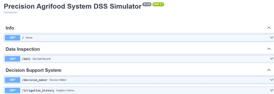
Figure 3.11 FastAPI interactive interface via Swagger UI: allows you to automatically explore, test, and document the RESTful endpoints exposed by the framework.
