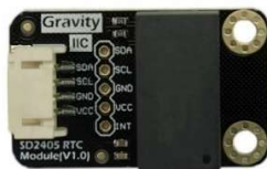
Figure 3.3 SD2405 RTC module with I 2 C interface and integrated rechargeable battery, for accurate date and time maintenance even without external power supply [40].
