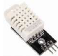
Figure 3.5 DHT22 digital sensor for precise measurement of air temperature and humidity.
