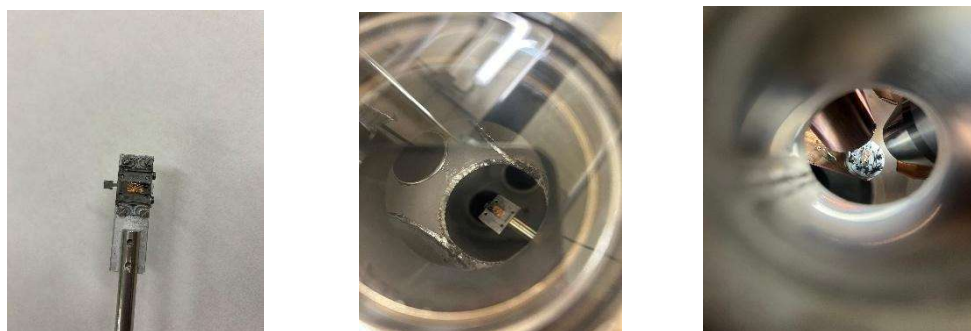
Figure 4.3.3 Images of the glass functionalized sample in XPS sample holder and XPS analysis chamber.
